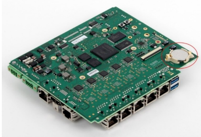
Figure 7: Location of RTC Battery on CPE400/CPL410/CPS400
