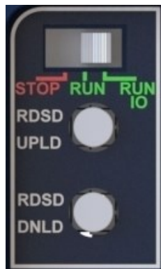
Figure 11: CPE330 Run/Stop Switch and RDSD Switches
